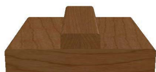
20 MINUTE: Veneered Engineered Wood or Fire core
