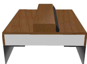
60 MINUTE: Veneered Fire Core (Shown with Optional Installation Angle Brackets)
